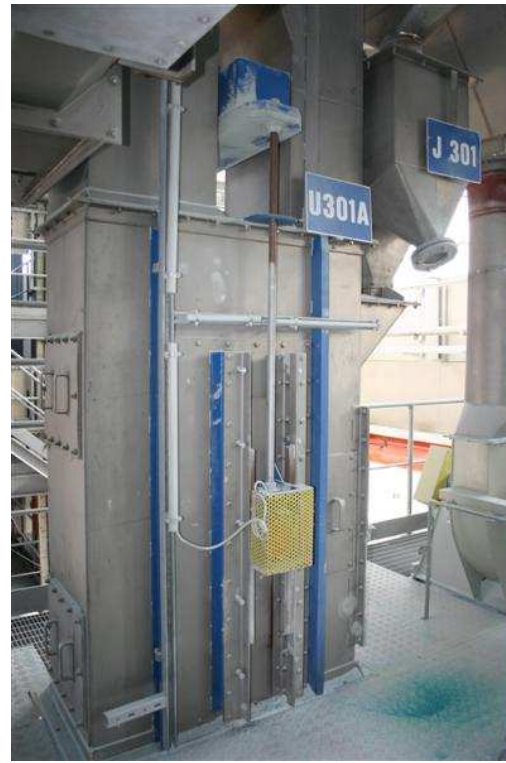
Samec Bucket Elevator ET 1000x600 – tension station
