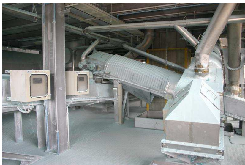
Samec Belt conveyor TN650 – weighing cell
