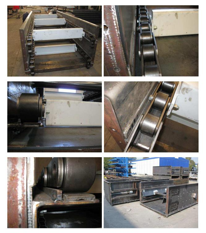
Plate chain and roller are both treatment to increase their wear protection. One case very 2 is equipment with lateral inspection windows needs to remove the joint link or look the internal condition of conveyor. The screws of blades fixing are extractible by the lateral windows.
